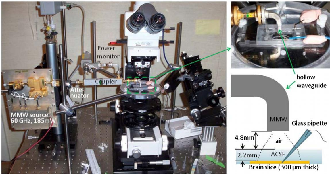
**Figure 1.** Left: electrophysiological setup with integrated MMW source. Right, top: close-up view of the tissue chamber and the hollow waveguide with an open-ended curved tip, allowing MMWs to be irradiated toward the tissue chamber. Right, bottom: schematic illustration of the MMW propagation from the tip of the waveguide. See the text for more details.
